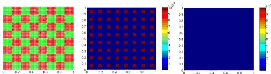
**Fig. 1.** Left: Coarse mesh. Center: Original coefficient. Here  $\eta = 10^9$ . Right: Coefficient  $\tilde{\kappa}$  computed as in (10) using (linear) multiscale basis functions.
