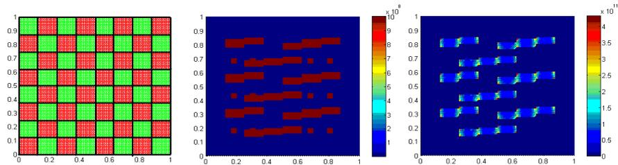
**Fig. 2.** Left: Coarse mesh. Center: Original coefficient. Right: Coefficient  $\tilde{\kappa}$  computed as in (10) using (linear) multiscale basis functions. The numerical results are presented in Table 1.
