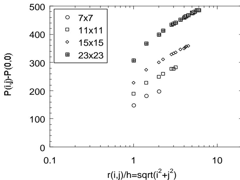
FIGURE 6. Numerical solution for pressure in a 5-spot well reservoir in the case of Forchheimer flow.
