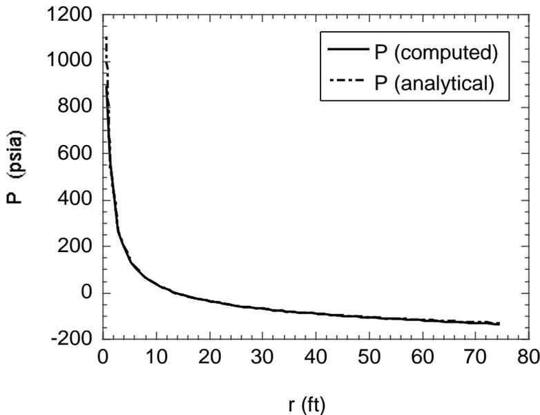
FIGURE 1. The computed and analytical normalized pressure for  $\beta = 1.71 \times 10^{11} ft^{-1}$ .
