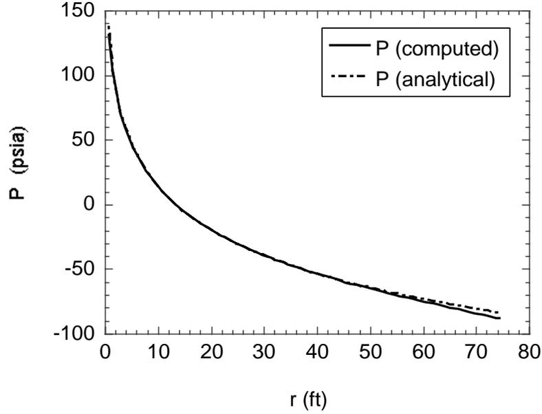
FIGURE 3. The computed and analytical normalized pressure for  $\beta = 0.0$ .
