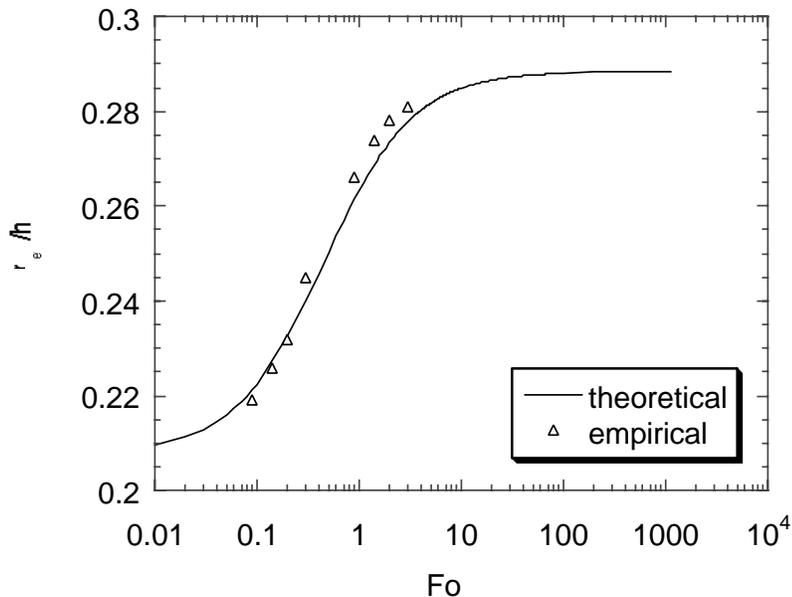
FIGURE 8. Dependence of  $\alpha$  on Forchheimer number and comparison of the graphically obtained  $\frac{r_{eff}}{h}$  for each Forchheimer number run with the theoretical curve (equation 3.11).
