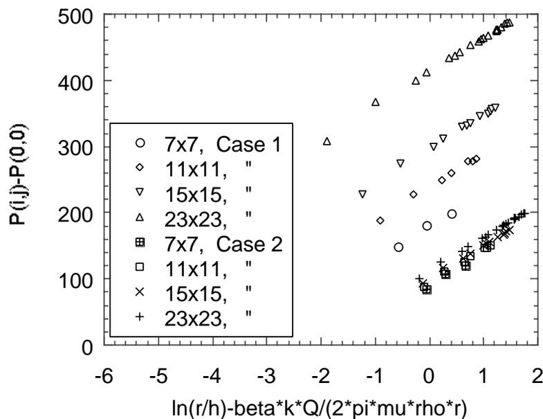
FIGURE 7. Numerical solution for pressure in a 5-spot well reservoir for Forchheimer flow. Case 1 is for  $\beta = 1.71 \times 10^{11} ft^{-1}$  and case 2 is for  $\beta = 1.71 \times 10^{10} ft^{-1}$
