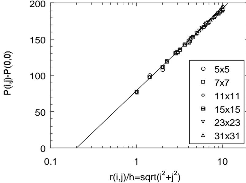
FIGURE 5. Numerical solution for pressure in a 5-spot well reservoir in the case of Darcy flow.
