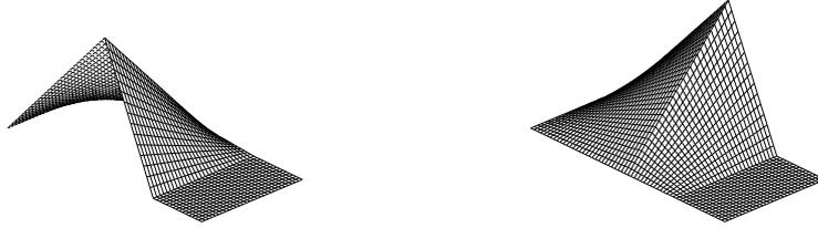
Fig. 10. “Condensed” shape functions for the adaptive mesh shown in Fig. 9.
