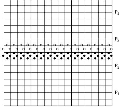
**Fig. 3.** Strip-wise data distribution between the processors.
