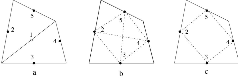
**Fig. 1.** (a) Node numbering of the super-element  $Q$ ; (b) Connectivity pattern of  $S_Q$ ; (c) Connectivity pattern of  $B_Q$ .
